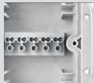
TOP IP66/IP67 version: integrated, one-piece gasket, fastening screws outside the gasket.
